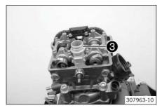
Remove the spark plug shaft insert 3.
