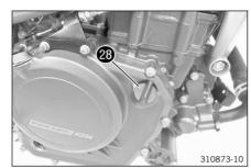
Remove filler plug 28 from the clutch cover together with the O-ring, and fill up with engine oil.
