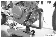
Position the floor jack under the engine and secure using the special tool.
