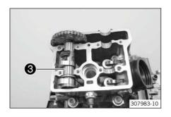
Remove exhaust camshaft 3.
