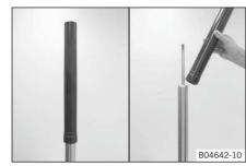
Remove the outer tube from the inner tube.
