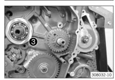
Mount timing chain sprocket 3.
