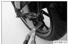
Press the brake piston back to its basic position and make sure that no brake fluid overflows from the brake fluid reservoir, extracting it if necessary.
