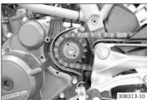
Position the engine sprocket in the chain and mount on the countershaft.
