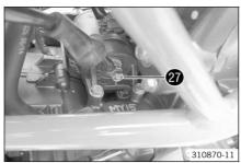
Mount and tighten nut 27 with the washers. Guideline
