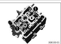
Check valve guides 1 with the special tool.
