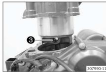
Feed the timing chain through the chain shaft. Mount piston pin 3.
