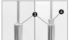
Tighten sliding bushing support 3 with special tool 4.
