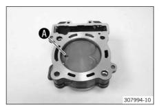
Ensure that piston marking A faces the outfeed side.
