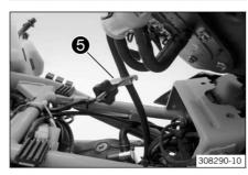
Detach the fuel line with a suitable tool 6.
