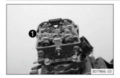
Mount and tighten the spark plug using special tool ①.
