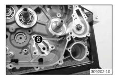
Position crankshaft to TDC and lock with special tool 6.
