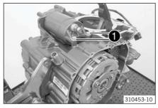
Grease the O-ring. Position the starter motor.
