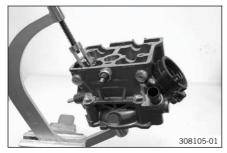
Tension the valve spring with a special tool.
