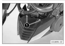
Position the front spoiler. Mount screws but do not tighten vet.
