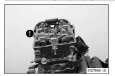
Remove the spark plug using special tool 1.
