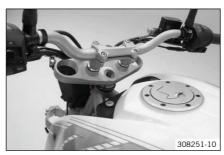
Remove the upper triple clamp with the handlebar and set aside.
