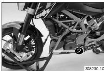
Mount special tool **2** on the left side of the vehicle.
