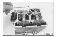
Remove the camshaft bearing bridge again. Compare the Plastigauge clearance gauge with the data on the packaging.
